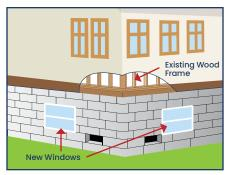
New foundation with flow-through openings.
