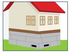
Finished foundation walls with flowthrough openings. House is lowered down on to the new walls.
