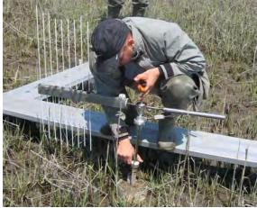
Figure 2. SET device temporarily installed to measure accretion rate at site, once measurements are taken the "head" is removed
