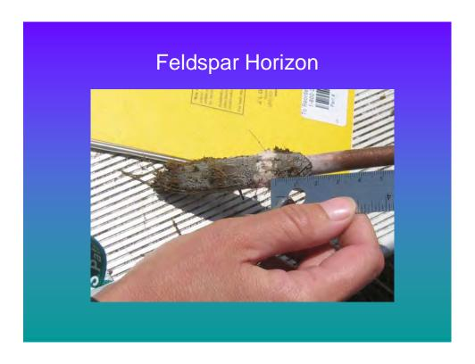
Figure 3. Feldspar companion measurement, measures amount of sediment deposited on marsh and compared to SET measurements, to check for marsh subsidence. A rod frozen with nitrogen is used to extract the sample from the marsh peat.
