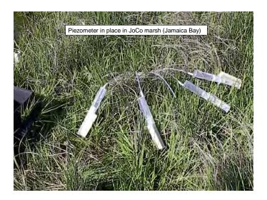
Figure 5. Suction devices used to collect pore water samples, these are removed and taken to the lab.
