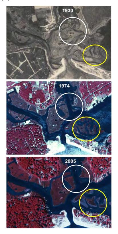
Figure 28. Channel and ditch widening on east side of North Sea Harbor
