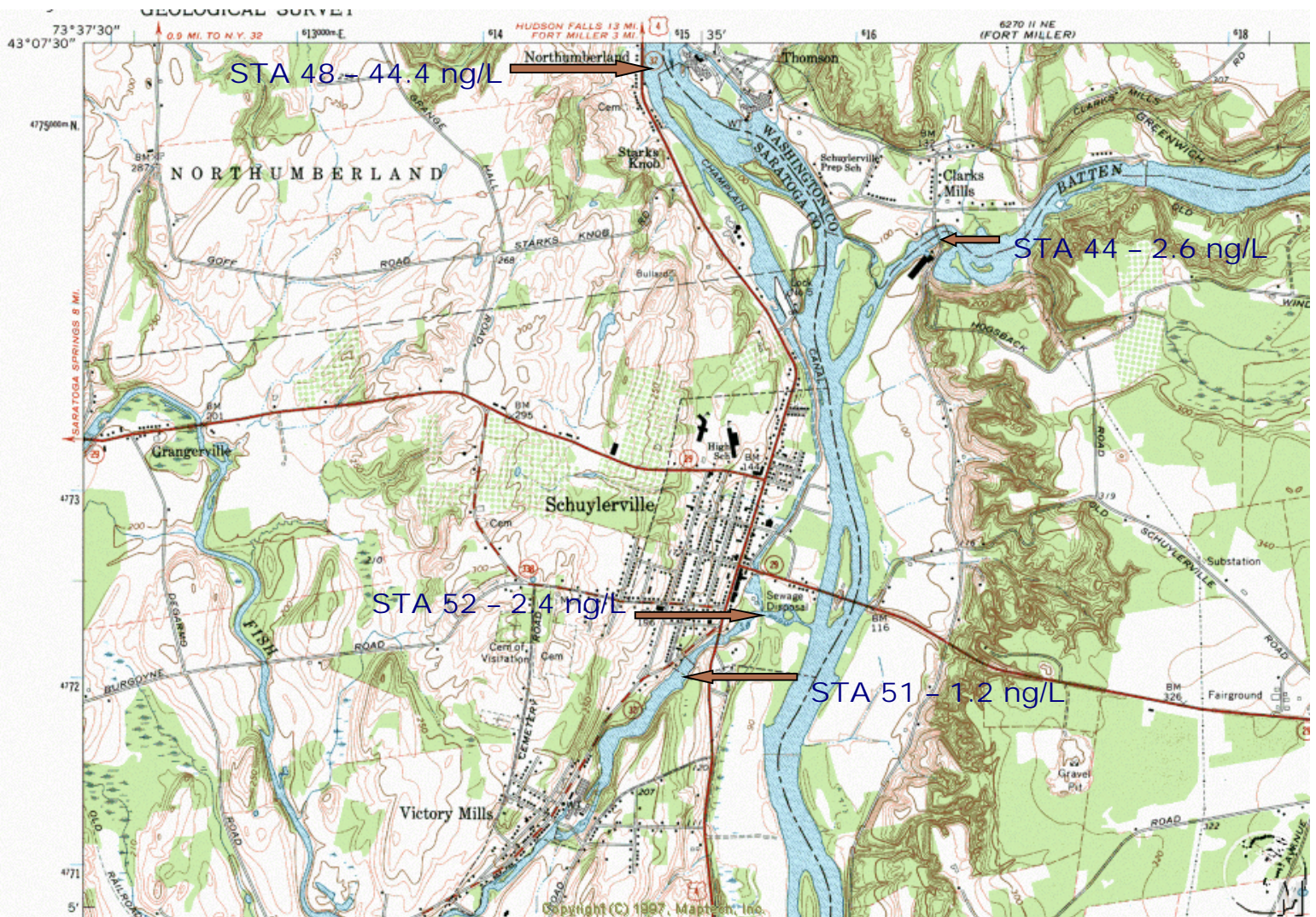
Figure No. 8. 1998 Upper Hudson River PISCES stations with results as PCB water concentrations (ng/L) – Schuylerville area stations.
