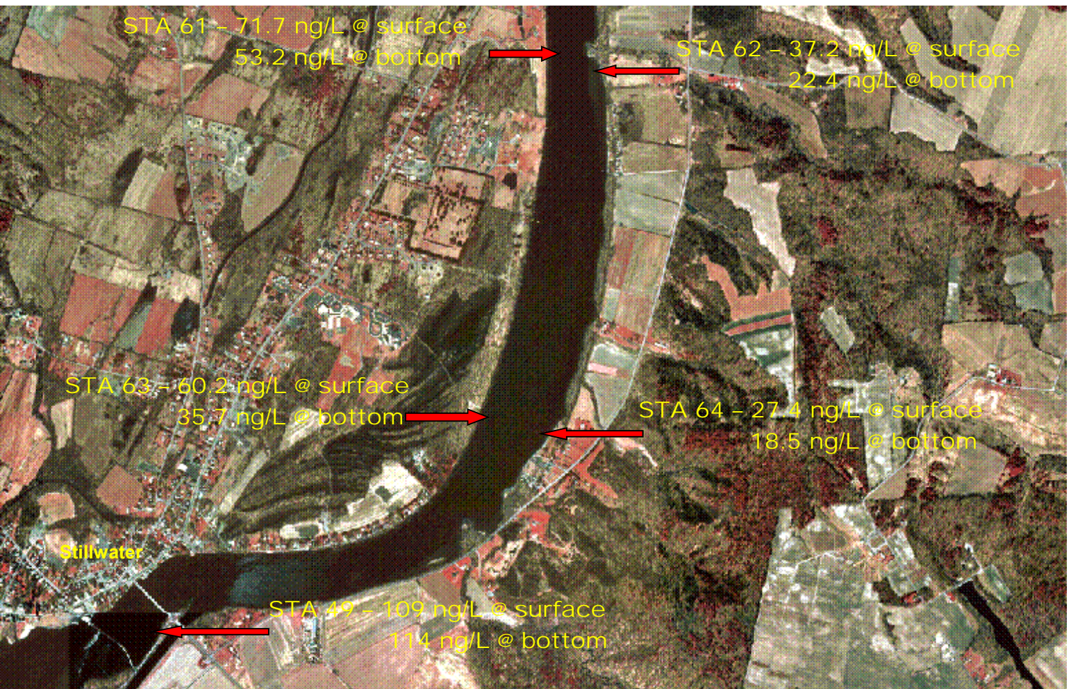
Figure No. 14. 2000 Upper Hudson River PISCES stations with results as PCB water concentrations (ng/L, analyses comparable to 1997/98) – Above the dam at Stillwater.
