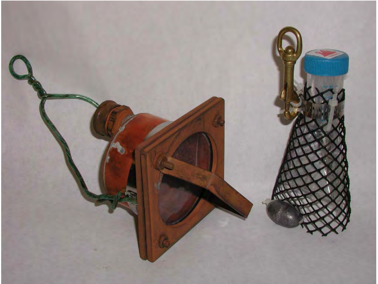
Figure 16. Types of passive samplers (PISCES) used in Upper Hudson River PCB trackdown; Hassett sampler (left) and bag sampler (right).
