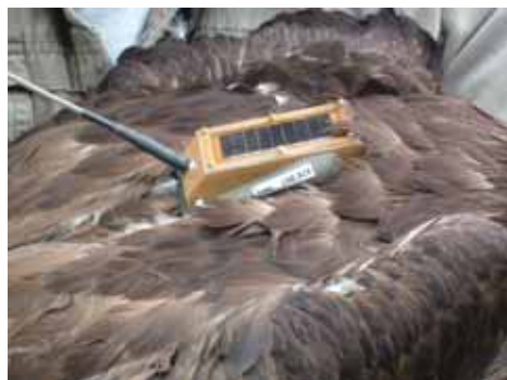
NY#19, Y90, Montezuma Refuge. Solar-powered backpack Ptt with blistered vhf radio Photo by: P.Nye
