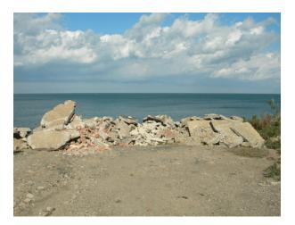
The above photo shows typical concrete rubble of greatly varying size. The larger slabs may not be suitable as filter layer material.
