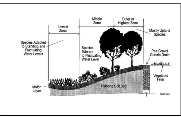
Figure H.1 Planting Zones for Bioretention Facilities
