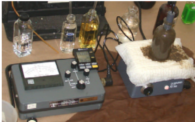
D.O. meter and probe, timer, 300 ml bottle and stir plate
