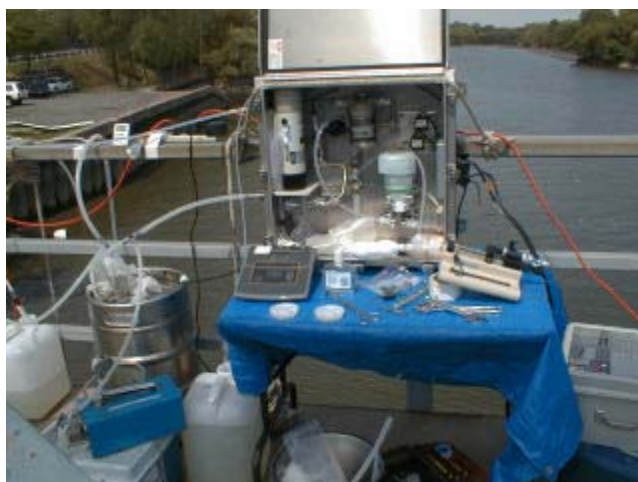
Figure 9. TOPS running on the Passaic River. Notice the stainless steel can on the left where large zooplankton are removed by filtration. A syringe pump delivering metered surrogates is seen on the table to the right of the TOPS. The plastic carboys on the deck collected water during timed intervals as an independent check of pumping rates. Note the lack of simplicity.
