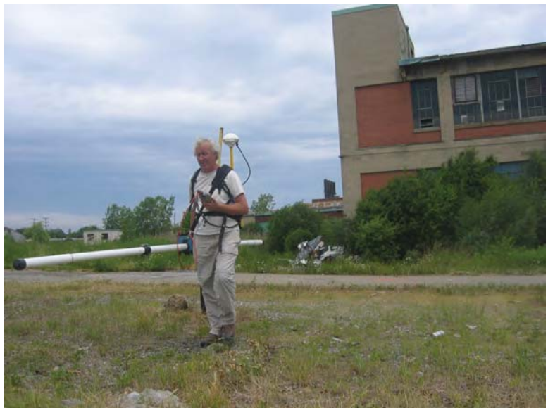
EM31 with GPS in use (photo not from this site)
