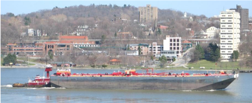
A tugboat pushes the RTC 120 past Poughkeepsie. The barge is empty, so it floats high in the water.
