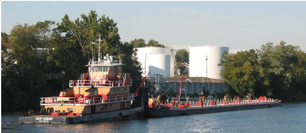
A tugboat brings a tanker barge to an oil tank farm in Troy. Since the barge is loaded with oil, it floats low in the water.
