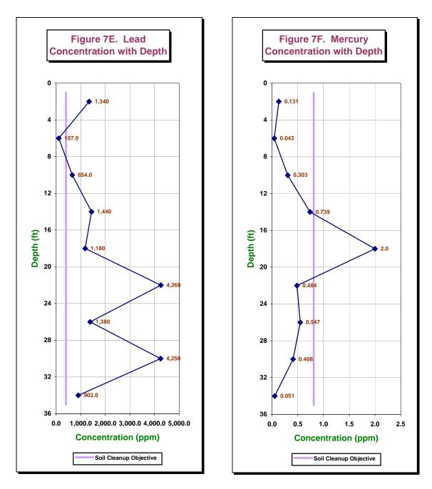
Figures 7E & F. Lead and mercury concentrations with depth in soil boring SB-2. The results are again plotted at the midpoint of the zone sampled.
