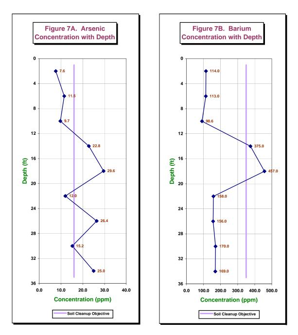
Figures 7A & B. Arsenic and barium concentrations with depth in soil boring SB-2. The results are plotted at the midpoint of the zone sampled (e.g., a sample collected from 28.0 to 32.0 feet depth is plotted at 32.0 feet).
