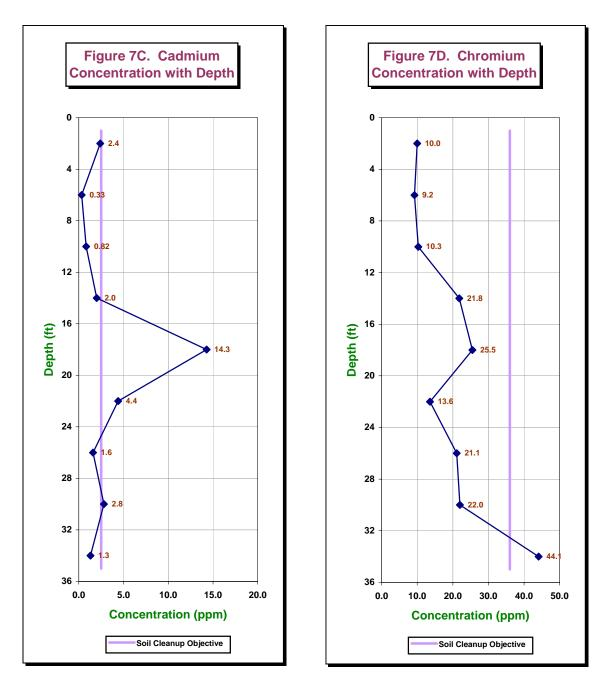
Figures 7C & D. Cadmium and chromium concentrations with depth in soil boring SB-2. The results are again plotted at the midpoint of the zone sampled.
