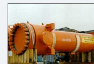
Industrial Example of a Tube & Shell Heat Exchanger
