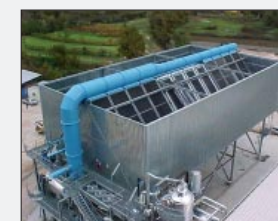
Industrial Example of a Finned Tube Heat Exchanger
