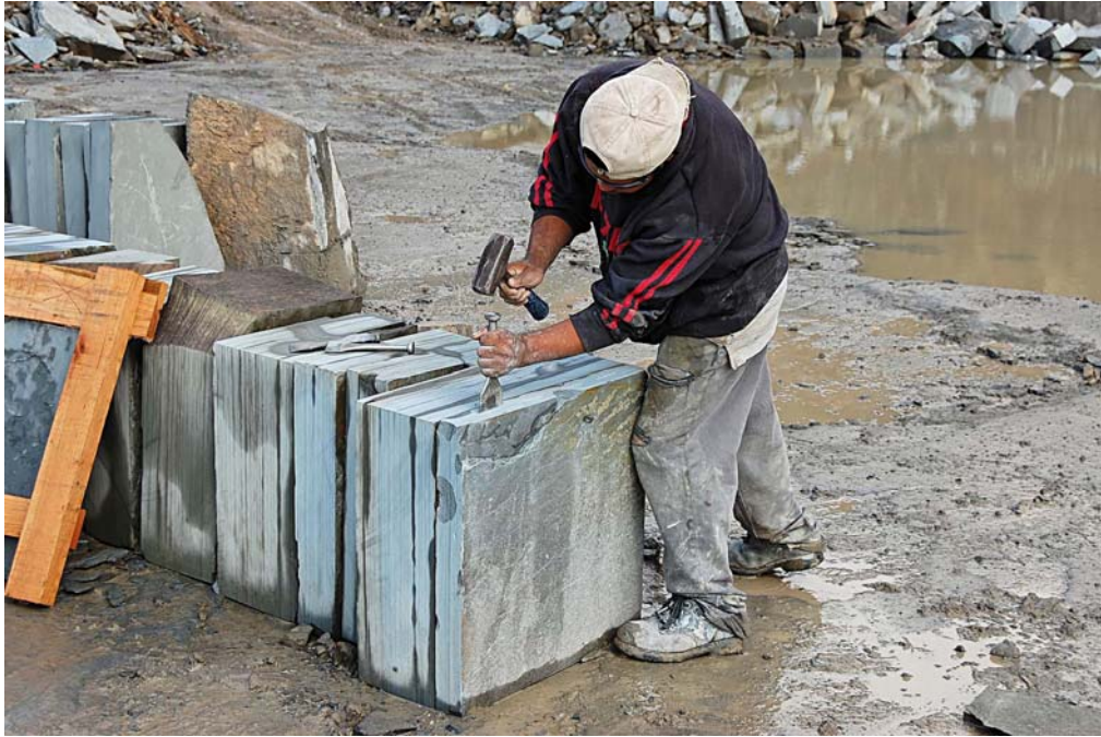
A worker at a bluestone mine demonstrates how bluestone can be broken into the slabs that make it such a popular landscaping and building material.
