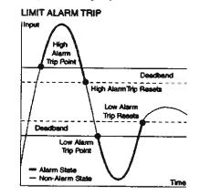
Figure 5. The SPA<sup>2</sup> can be used as a simple on/off controller such as those required in level applications (pump/valve control) when filling or emptying a container or tank.
