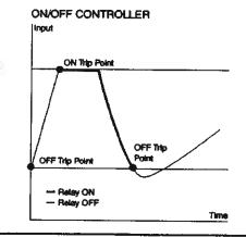
Figure 6. The SPA<sup>2</sup> can be set to trip when the input rale-of-change exceeds a user-selected rate (Delta) over a user-selected time period (Delta Time).
