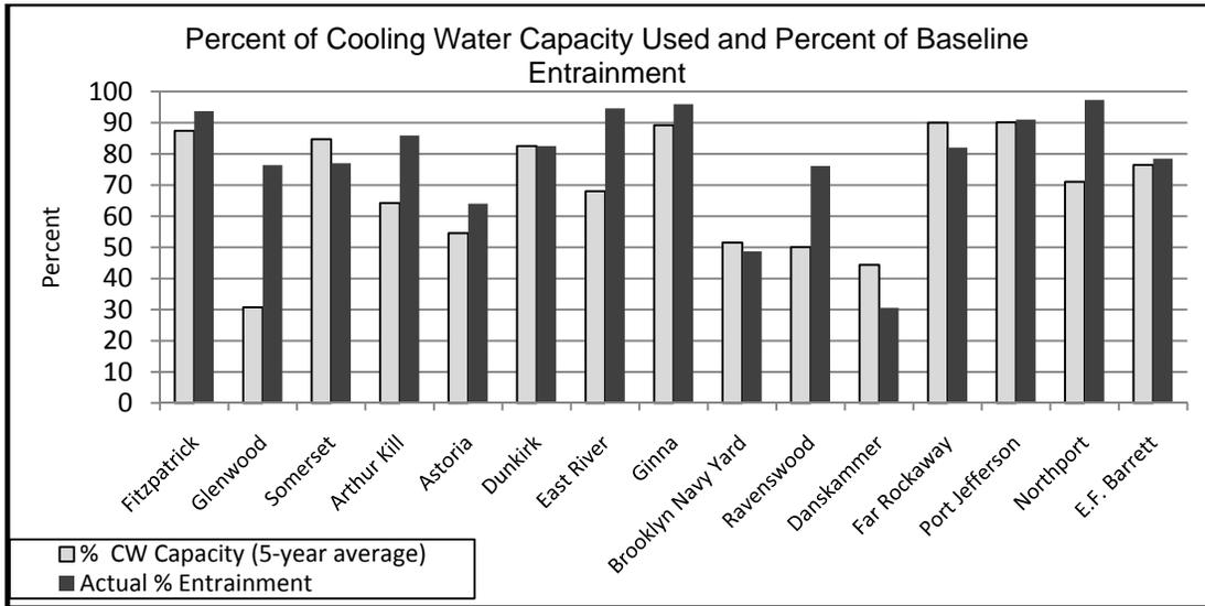
Figure 7: Percent cooling water capacity used and percent of baseline entrainment at 15 steam electric facilities in New York.
