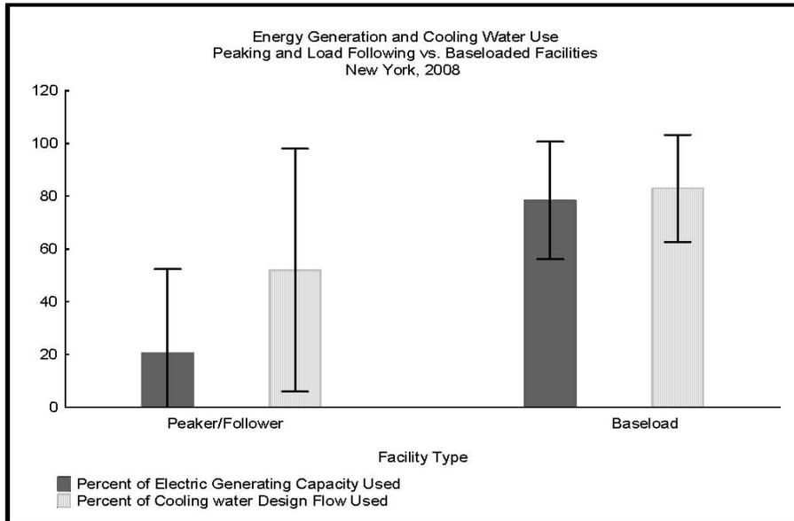
**Figure 5: Average electric generating capacity and cooling water capacity utilization at peaking and load-following vs. baseloaded steam electric facilities in New York State during 2008. Error bars represent +/- 2 STD.**
