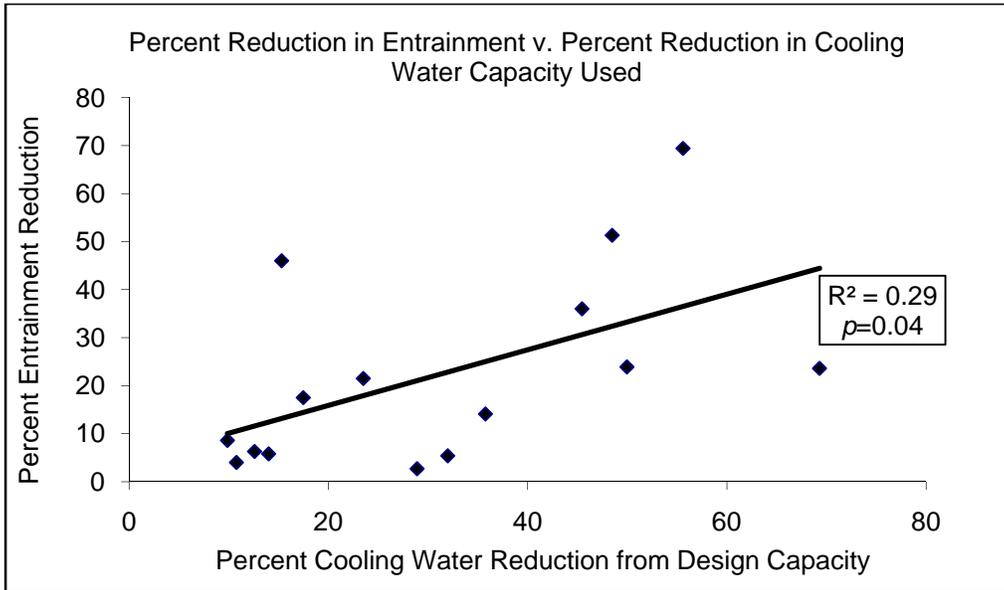
**Figure 2: Reductions in entrainment from baseline conditions as a result of reducing cooling water use at 15 steam electric facilities in New York State. Though the relationship is predictably positive, only 29% of the variability can be attributed to reductions in cooling water use. Over 70% of the variability is likely due to the strong seasonality of ichthyoplankton density and energy demand.**
