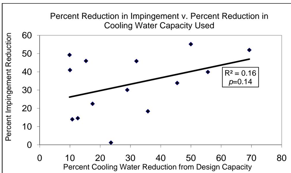
**Figure 1: Reductions in impingement from baseline conditions at 14 steam electric facilities in New York State compared with cooling water reductions. The weak relationship is likely due to the effectiveness of traveling screens and fish return systems at some of these facilities in reducing the impingement of many fish species. Seasonality of fish abundance and electric generating demand also likely influence these results.**
