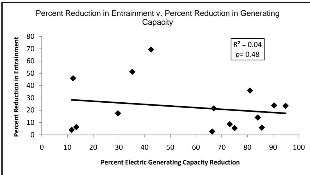
Figure 8: Regression between the percent reduction in entrainment from baseline conditions and the percent reductions in electric generating capacity used. Though not significant, the general relationship indicates that steam electric facilities in New York State utilizing the least amount of electric generating capacity have minimally reduced entrainment from baseline conditions.
