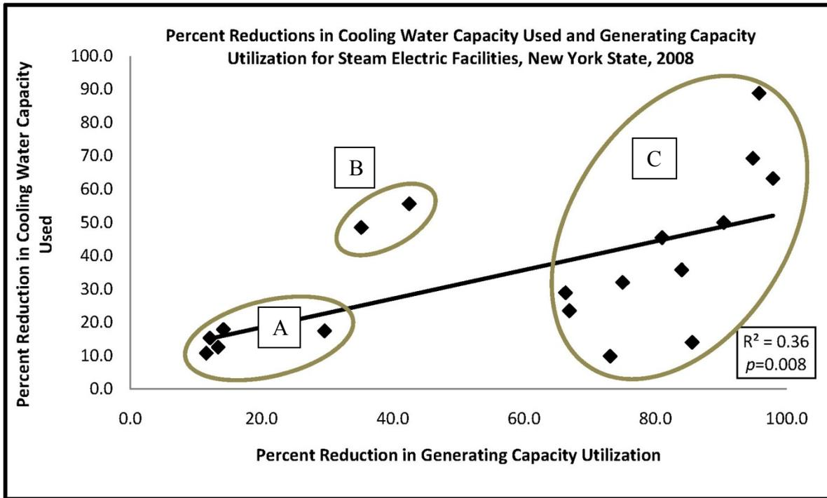
**Figure 4: Relationship between the reduction in cooling water capacity used as a function of reducing electric generation at 18 steam electric facilities in New York. The groupings correspond to generating operations (A=baseloaded; B=unique water use; C=peaking and load-following facilities).**
