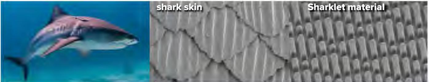
Shark skin scales (denticles) are arranged in a distinct diamond pattern with tiny bumps that prevent algae from growing and that pattern when used on other surfaces such as plastic also keeps bacteria from growing too! By mimicking the pattern of the shark skin scales, a company called Sharklet Technologies is creating products that are able to keep bacteria from growing on different surfaces. This is helping to prevent people from getting sick.
