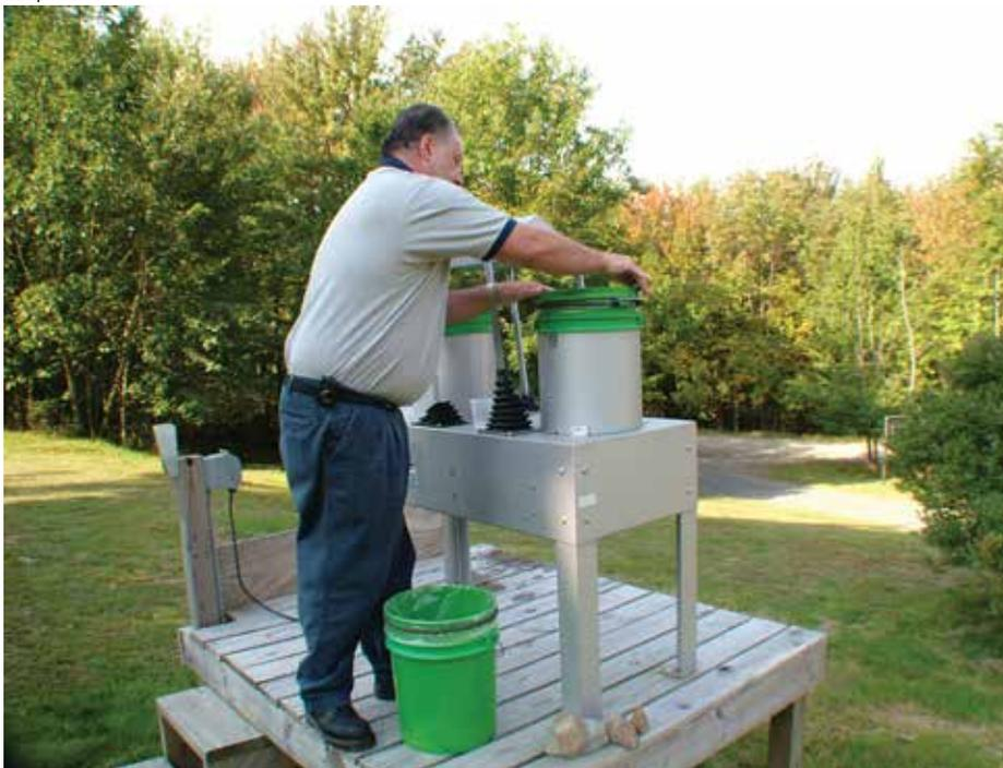
A DEC staffer checks the equipment at one of the acid rain monitoring stations.
